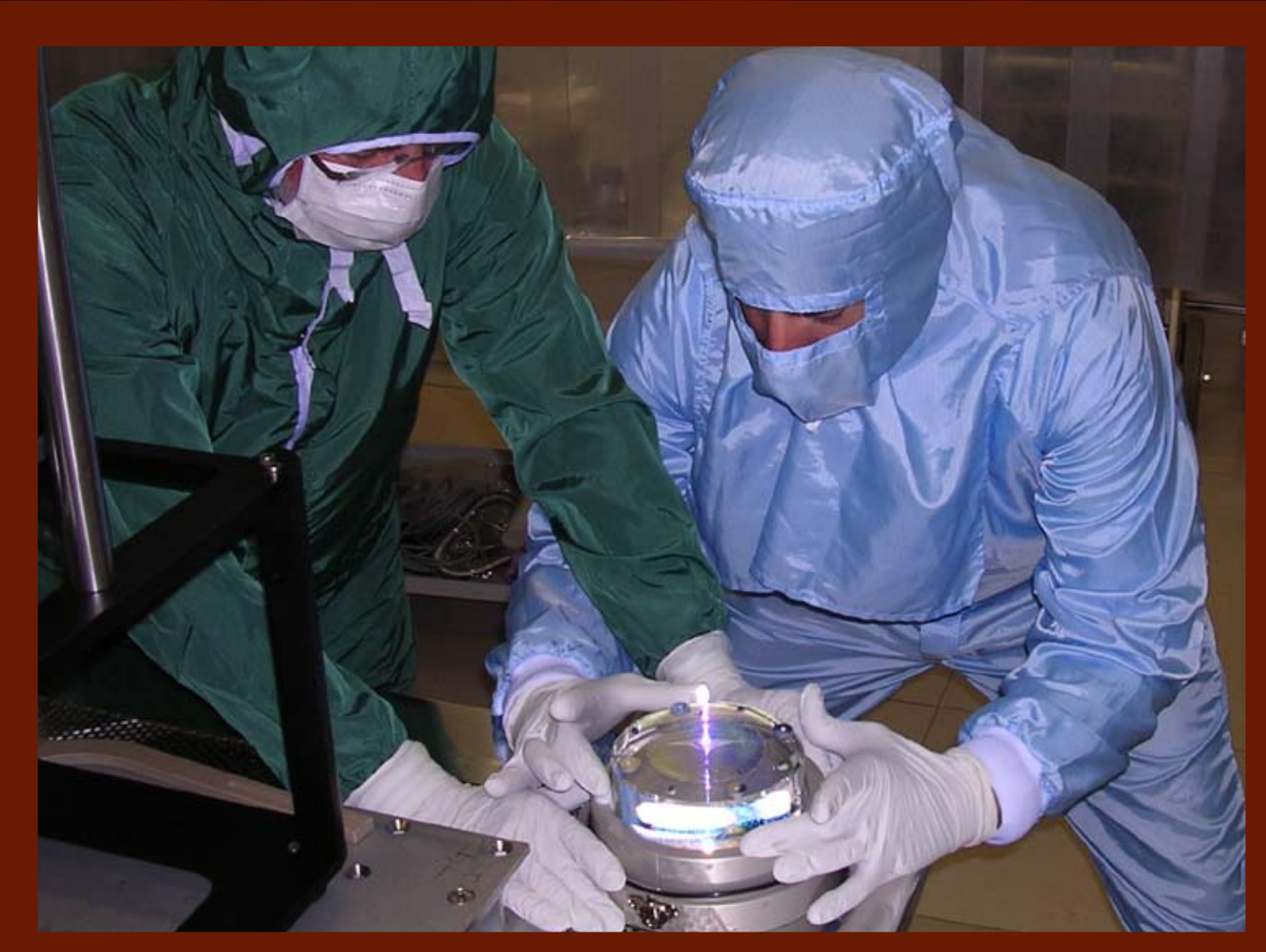
Installation of advanced new optics by Nikhef personnel for the Virgo+ upgrade.
