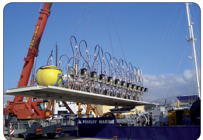
Fig. 2. The platform carrying the first detector line of ANTARES is loaded onto the sea vessel 'CASTOR', prior to its deployment in the Mediterranean Sea.
