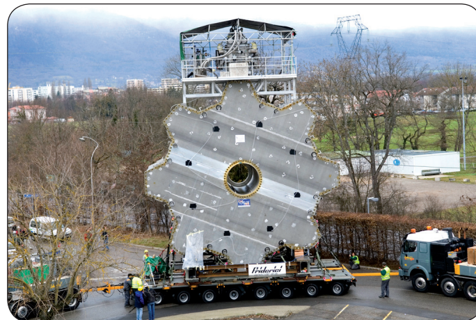
Fig. 6. An ATLAS endcap toroid magnet in its cryostat is transported at CERN.
