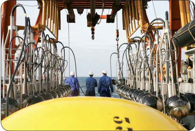
Fig. 3. ANTARES lines waiting to be lowered into the sea.
