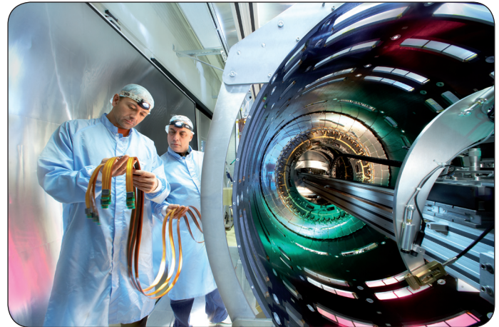
Fig. 1. Nikhef technicians working on the Silicon Tracker (SCT) for ATLAS.
