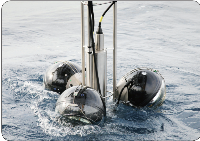
Fig. 3. Deployment of one of the 25 stories of the first ANTARES detector line. A story is seen to consist of three glass spheres each housing a large photomultiplier tube. At the centre of each story a titanium cylinder contains all readout and control electronics.
