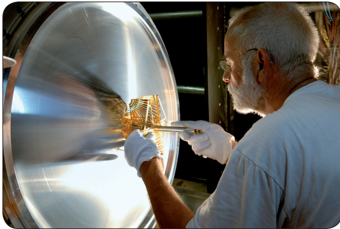
Fig. 3. Installation at CERN of the wakefield suppressor on the VELO setup.
