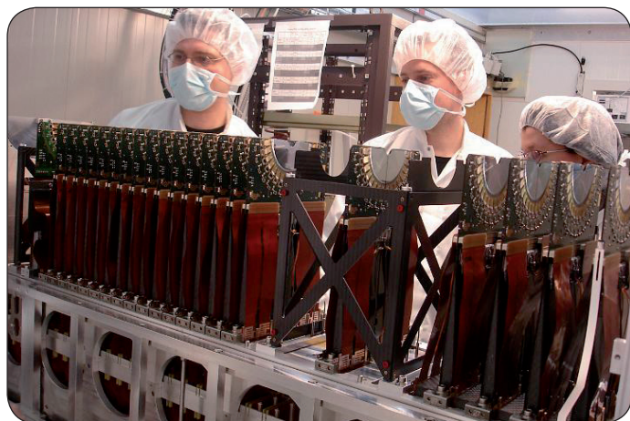
Fig. 2. The VELO and Pile-Up detector modules as installed in the first half detector.
