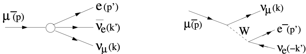
Figure 7.2: Muon decay: left: Labelling of the momenta, right: Feynman diagram. For the spinor of the outgoing anti-particle we use u_{\nu_e}(-k') = v_{\bar{\nu}_e}(k') .
