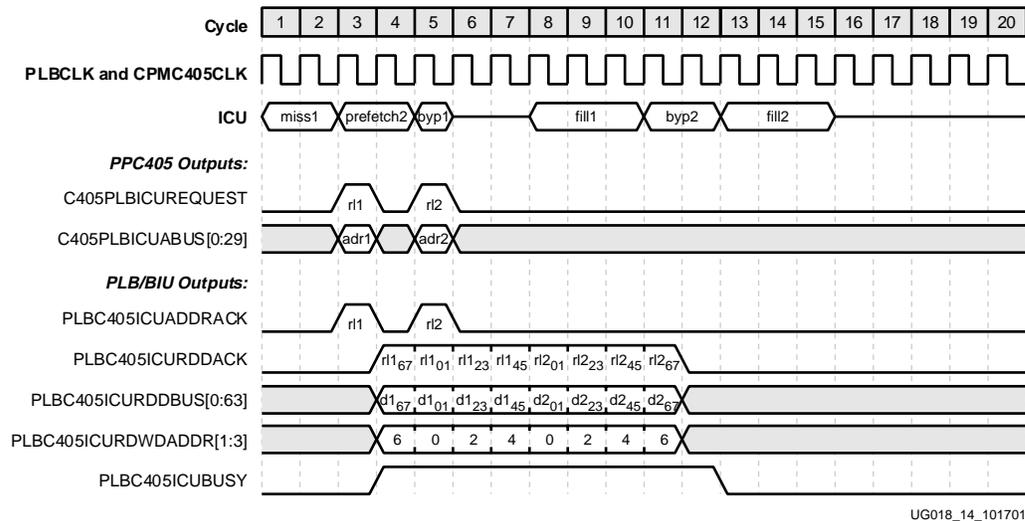
Figure 2-9: ISPLB Pipelined Cacheable Sequential Fetch (Case 2)
