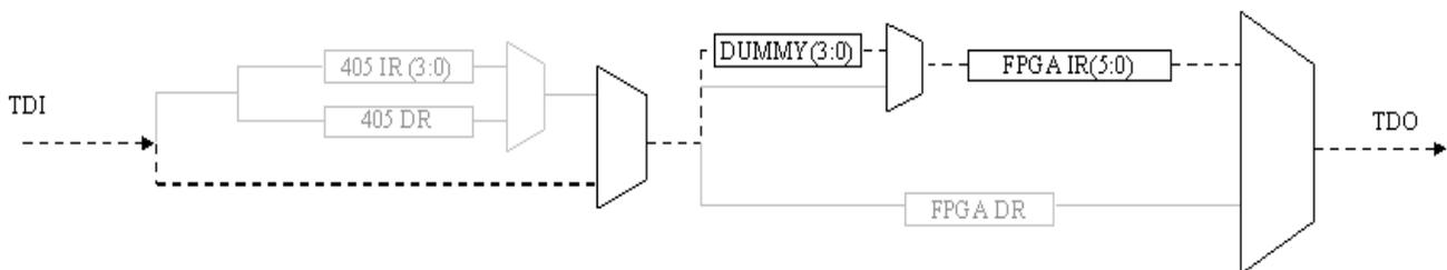
**Figure 2-39: Default Virtex-II Pro Instruction Register data path (XC2VP4, XC2VP7)**
