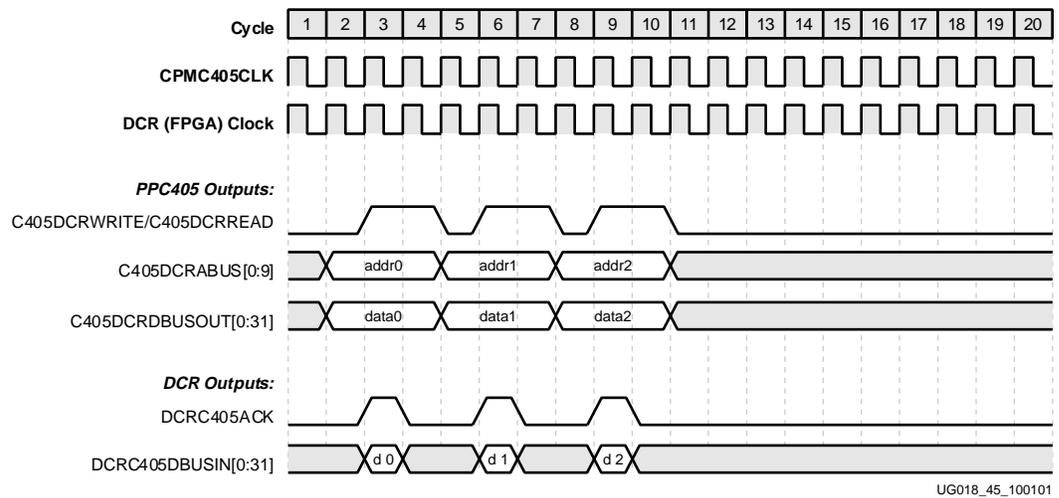
Figure 2-36: DCR Interface Mode 1, 1:1 Clocking, Combinatorial Acknowledge
