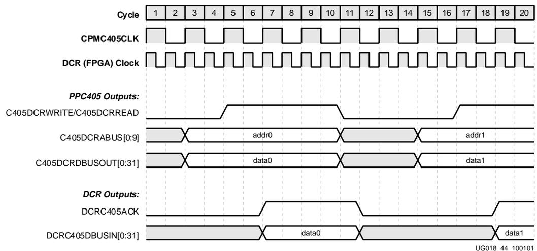
*Figure 2-35: DCR Interface Mode 0, 1:2 Clocking, Latched Acknowledge*
