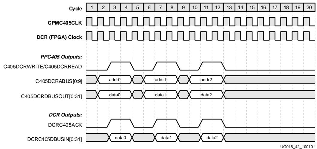
Figure 2-33: DCR Interface Mode 0, 1:1 Clocking, Combinatorial Acknowledge
