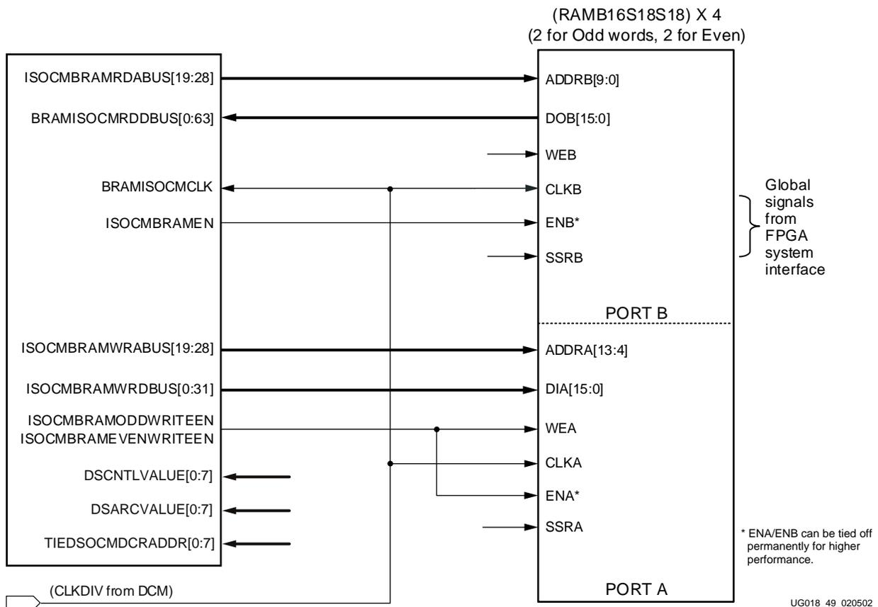
Figure 3-4: ISOCM to BRAM Interface: 8K Example
