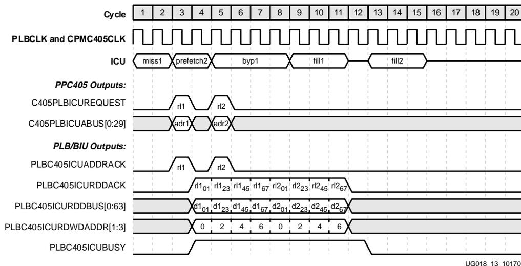
Figure 2-8: ISPLB Pipelined Cacheable Sequential Fetch (Case 1)
