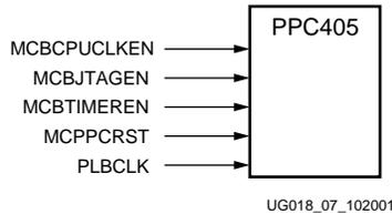
Figure 2-48: FPGA-Specific Interface Block Symbol
