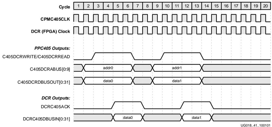
Figure 2-32: DCR Interface Mode 0, 1:1 Clocking, Latched Acknowledge
