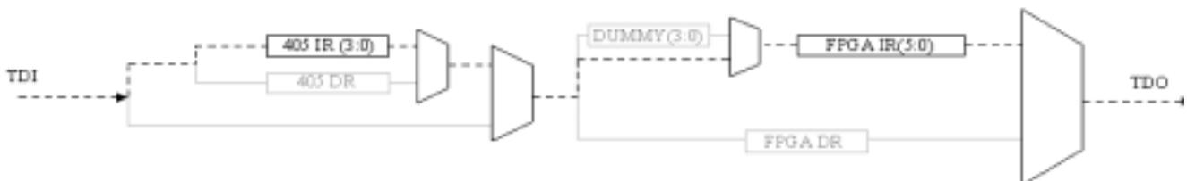
**Figure 2-40: Virtex-II Pro Instruction Register data path for Series PPC405 JTAG connection (XC2VP4, XC2VP7)**
