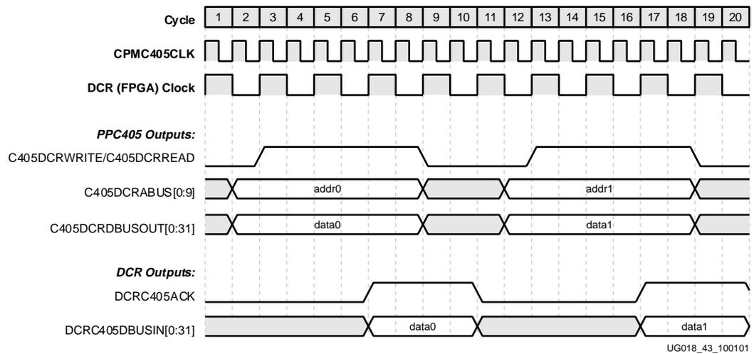
Figure 2-34: DCR Interface Mode 0, 2:1 Clocking, Latched Acknowledge
