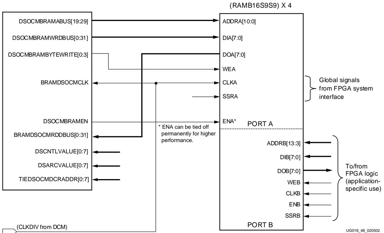
Figure 3-2: DSOCM to BRAM Interface: 8K Example
