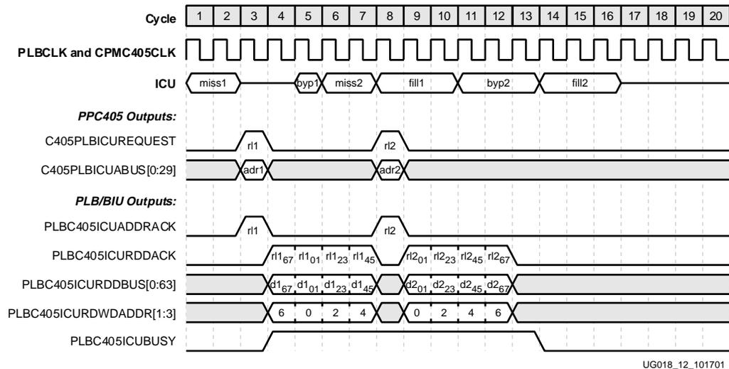
Figure 2-7: ISPLB Non-Pipelined Cacheable Sequential Fetch (Case 2)
