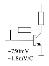
We use a dummy input diode as temperature sensor (Not callibrated yet)
