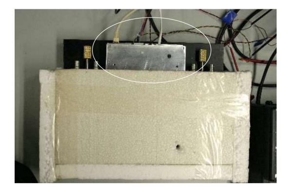
The Front Ends of the Outer Tracker are closely packed, heat must be extracted with cooling water along the Aluminium cooling extension plate. For the test we use a cooling block with forced air Several sensors monitor heatup of components.
