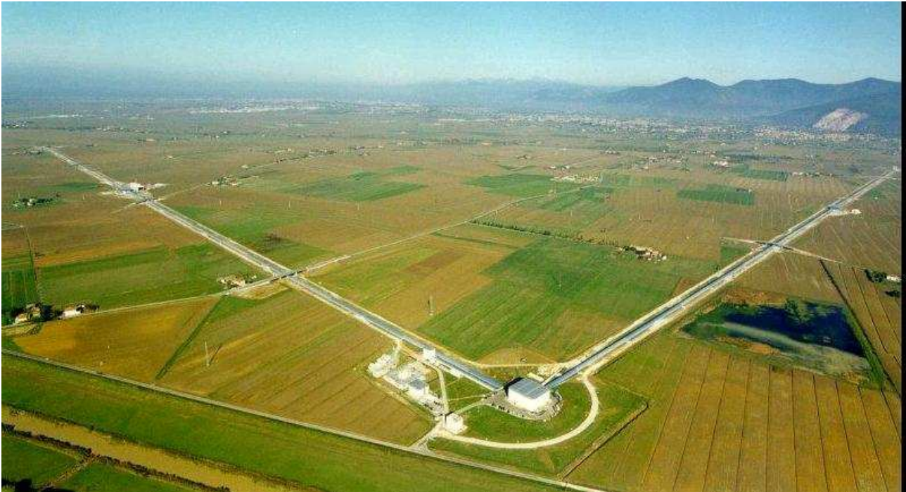
Figure 1: Aerial view of the VIRGO interferometer near Pisa, Italy. It consists of two 3 km long arms.
