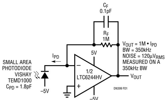
**Figure 1. Transimpedance Amplifier for Small Area Photodiode**
