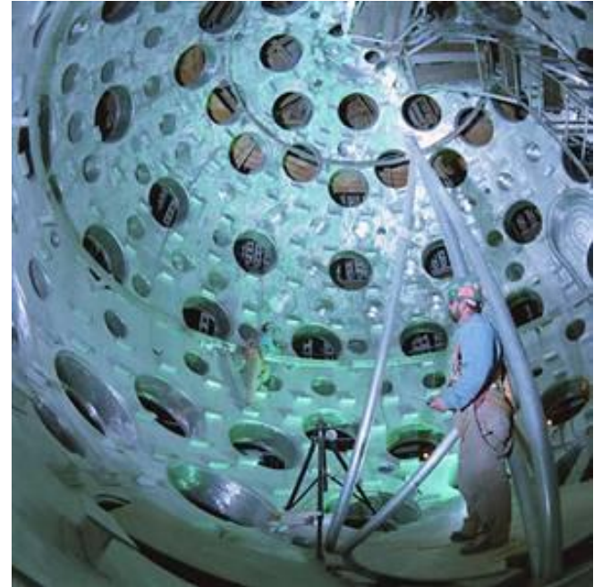
Target chamber, NIF with 192 laser beams
