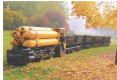
Figure 20.24. Top: A compressed-air tram taking on air and steam in Nantes. Powering the trams of Nantes used 4.4 kg of coal (36 kWh) per vehicle-km, or 115 kWh per 100 p-km, if the trams were full. [5qhvcb] Bottom: A compressed-air locomotive; weight 9.2 t, pressure 175 bar, power 26 kW; photo courtesy
