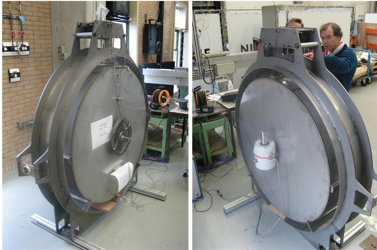
Figure 7: Photographs of the test stand for measuring the attenuation performance of the suspension system envisioned for the cryolinks of Advanced Virgo.
