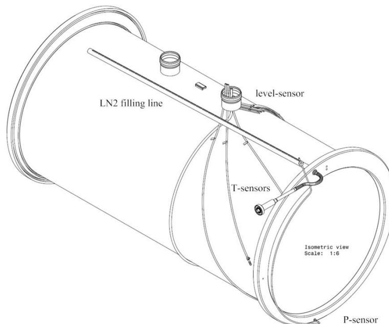
**Figure 8:** Schematic view of part of the sensors for the cryolinks.
