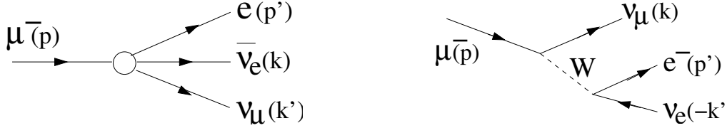
Figure 7.1: Muon decay: left : Labelling of the momenta, right : Feynman diagram. For the spinor of the outgoing anti-particle we use u_{\nu_e}(-k') = v_{\nu_e}(k') .
