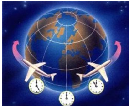
Figure 3.4: Atomic clocks were synchronized and taken on board of planes flying eastward and westward around the earth. After arrival they were compared and the prediction of relativity was seen to be correct.
