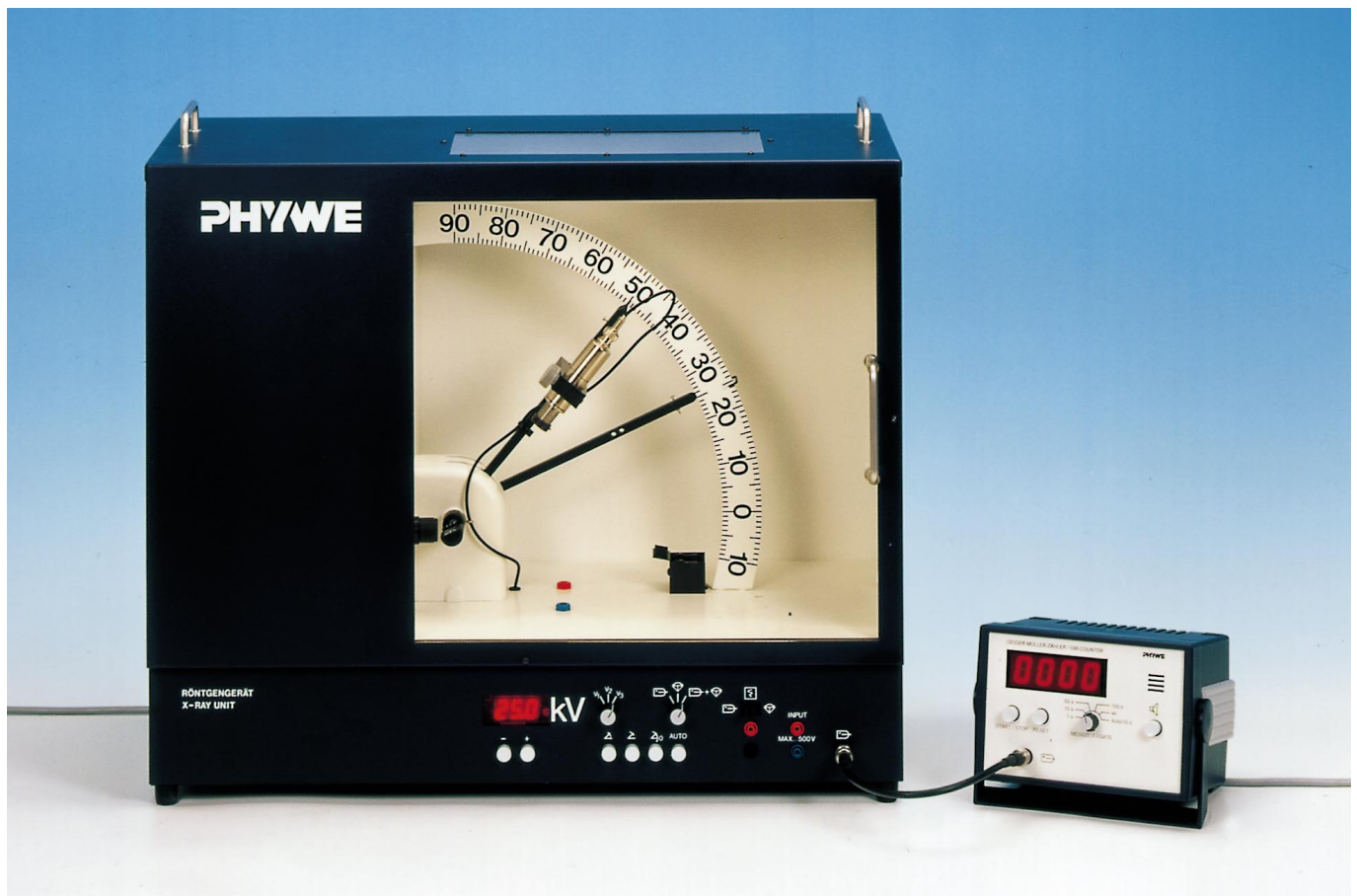
Fig. 1: Experimental set-up for determining the intensity of X-radiation as a function of the anode voltage.
