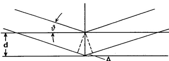
Fig. 4: Bragg scattering on the lattice planes.
