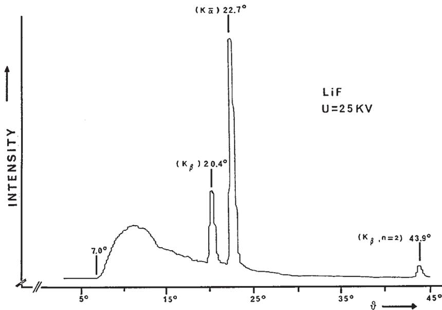
In order to obtain exact angle determination of the brems-spectra, the sensitivity of the x-channel must be increased accordingly and calibrated carefully; likewise, the zero-line of the y-axis must be displaced for each new measurement.
