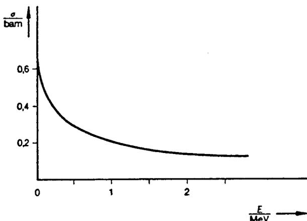
Fig. 2: Cross-section for the Compton effect  $\sigma_C$  in accordance with the Klein-Nishina equation.
