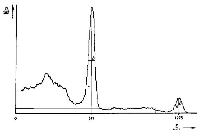
Fig. 4:  $\gamma$ -spectrum of  $^{22}\text{Na}$ .
