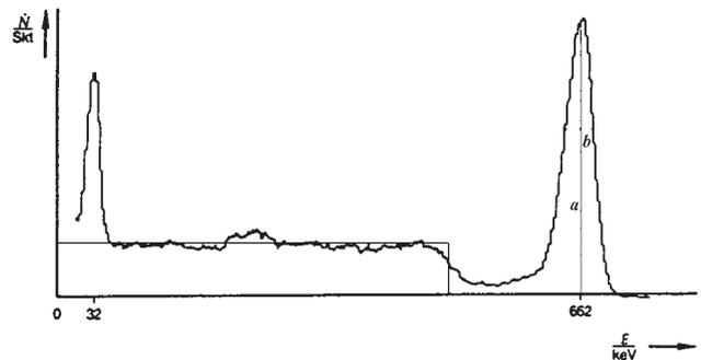
The Compton-scattered fraction in a  $\gamma$ -spectrum is represented by a continuous plateau which extends from the energy 0 to a steep fall at the Compton border; the electrons detected here are generated by a central impact and entrain the maximum possible energy. The area portions in the spectrum provide a direct measurement of the occurrence of the particular effect.
