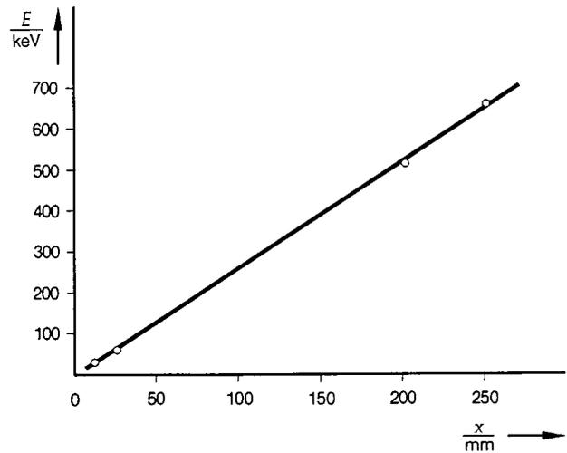
1. The set-up is calibrated by recording peaks of known energy: Cs-137, Am-241 and Na-22. Plot the energies on a graph as a function of the position of the xyt recorder ( $x$ ). Determine the slope either graphically or by linear regression with the expression  $E = a + bx$ . Using the values from Fig. 6, this gives:
