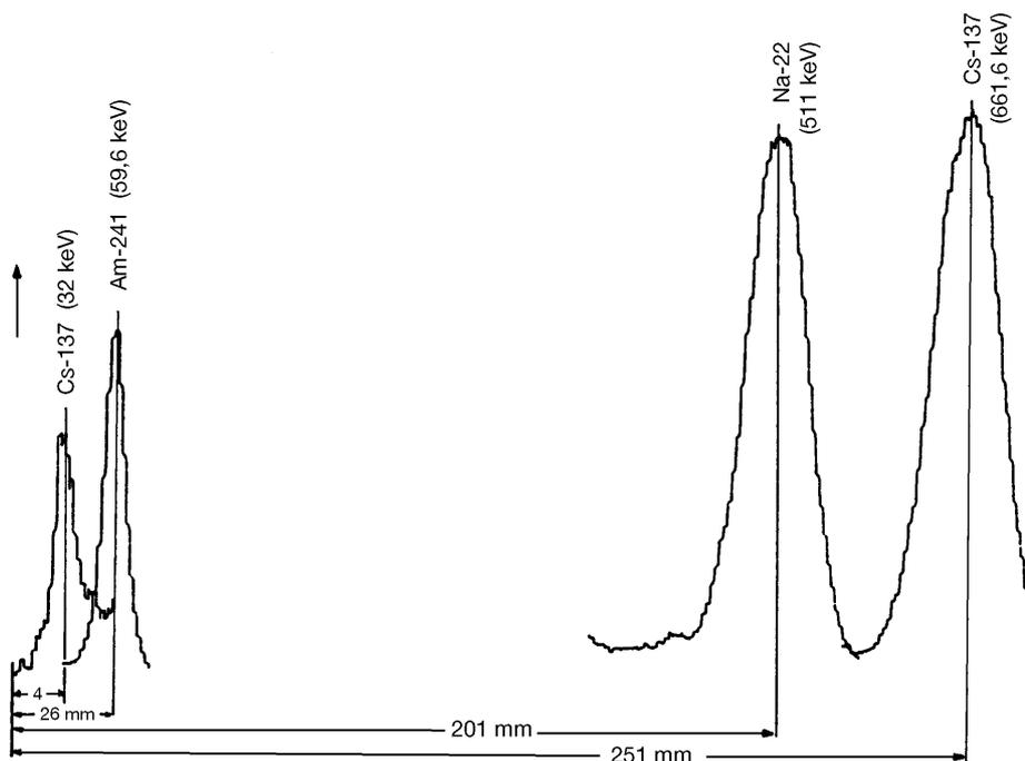
Fig. 5: Energy of known peaks as a function of the position of the xyt recorder.
