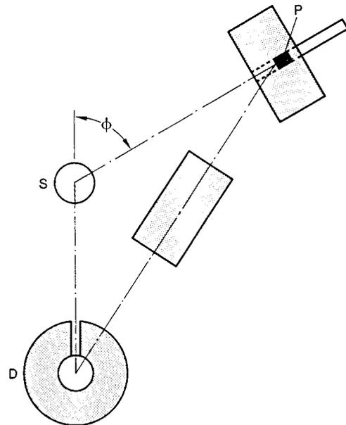
The positioning of the lead brick is crucial, in that Compton scattering also occurs in the lead. If necessary, try out several positions.
