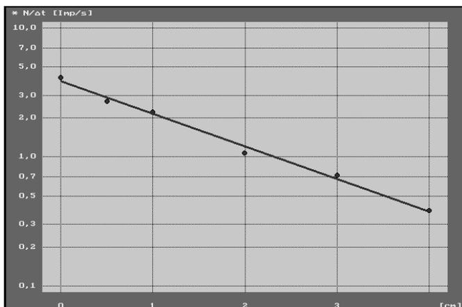
Fig. 2: Logarithmed counting rate (Co-60) as dependent on the absorbing film thickness (Pb)
