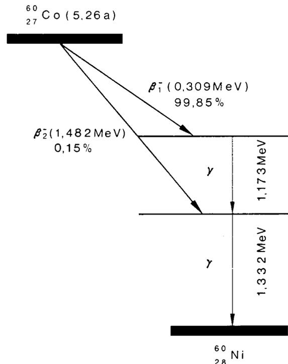
Fig. 3: Term diagram of  $^{60}_{27}\text{Co}$ .
