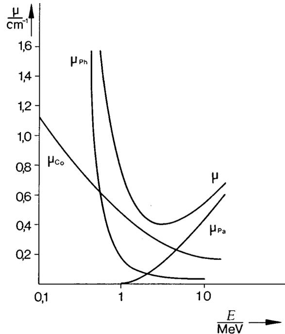
Fig. 6: Absorption of gamma rays by leads as a function of the energy ( $\mu_{Co}$  = fraction due to Compton effect,  $\mu_{Ph}$  = fraction due to photoelectric effect,  $\mu_{Pa}$  = fraction due to pair formation). The total absorption coefficient (attenuation coefficient) is  $\mu = \mu_{Co} + \mu_{Ph} + \mu_{Pa}$
