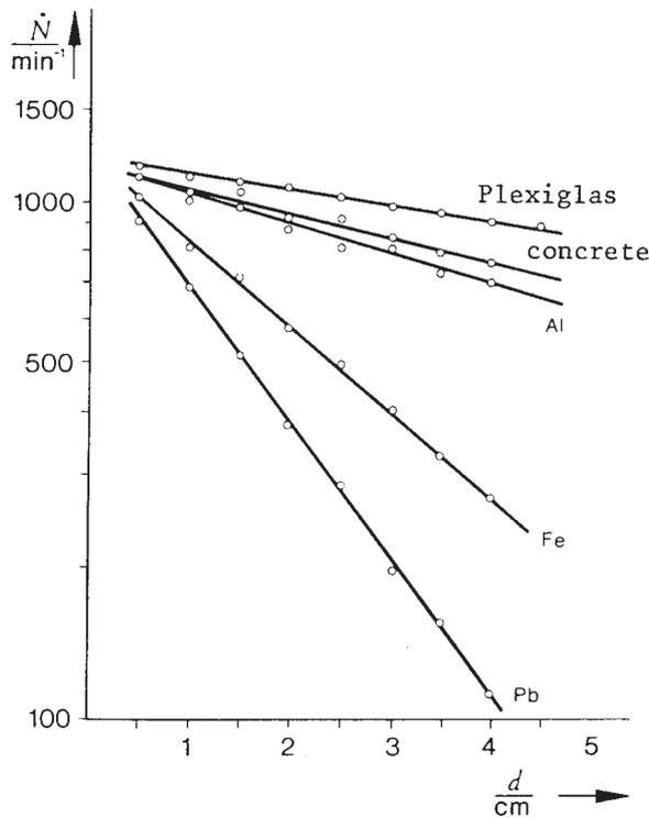
We can see from the  $\mu/E$  curves in Fig. 7 that lead is particularly suitable as an absorber of gamma rays of low or high energy.
