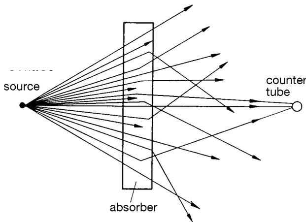
from a point at the centre of the counter tube. Then determine the background radiation  $\dot{N}_0$  without the preparation and subtract it from the measured counting rates  $\dot{N}'(r)$ :
