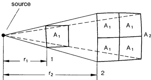
The reason for this is that, as shown by Fig. 4, the area of a sphere round the source through which a beam of rays passes, increases as the square of the distance  $r$ . In vacuum (in air), therefore
