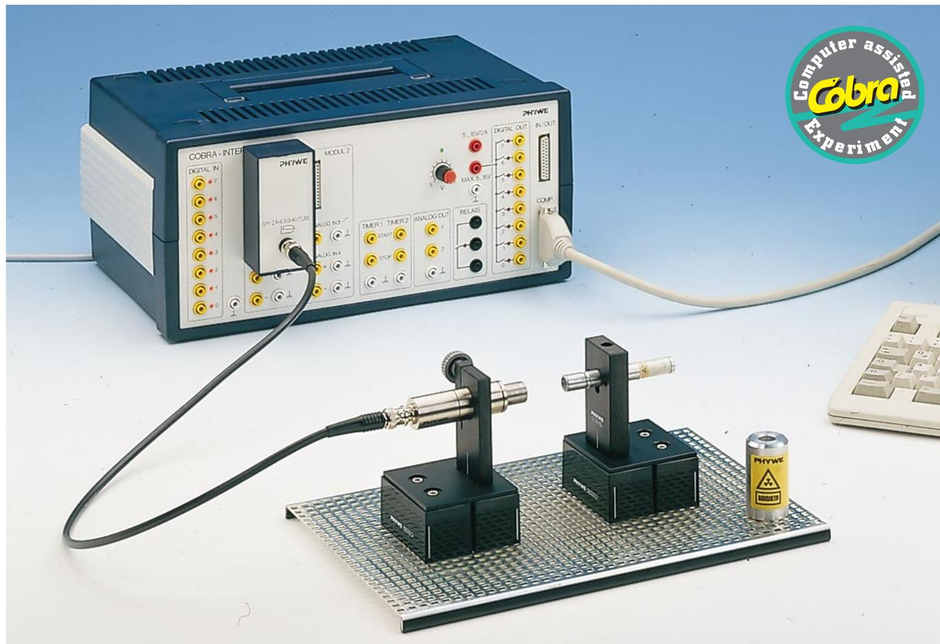
— Check the measured value. If necessary, change the gap between the radioactive source and the counter tube in order to obtain the desired number of counts. To get low pulse rates, it will be helpful to put a sheet of paper between the source and the counter tube.
