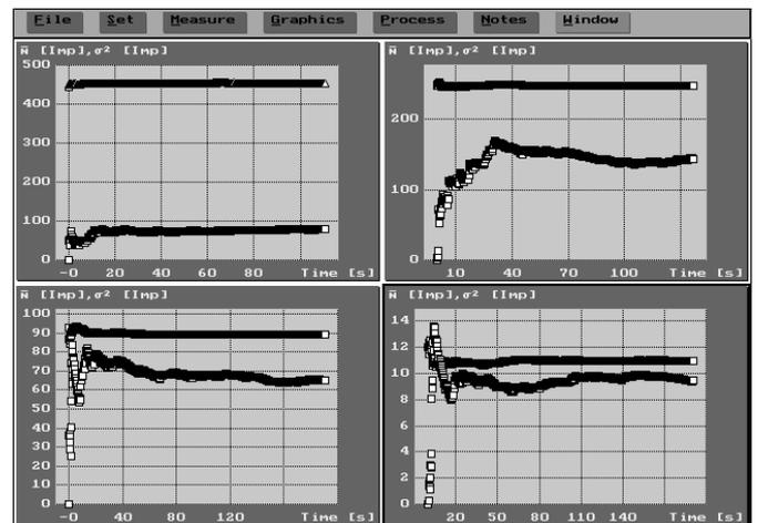
Fig. 3: Mean value and variance in the case of average pulse rates of 4600, 2500, 900 and 110 pulses/s.
