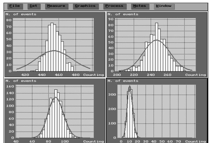
Fig. 4: Statistical distribution for average pulse rates of 4600, 2500, 900 and 110 pulses/s compared to the theoretical Poisson's distributions.
