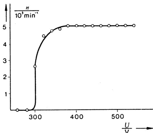
Fig. 5: Counting rate at constant activity, as a function of the counter tube voltage.
