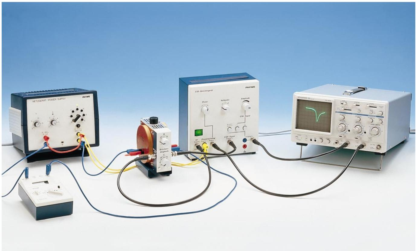
Fig. 2a: Measuring bridge of the ESR apparatus.
