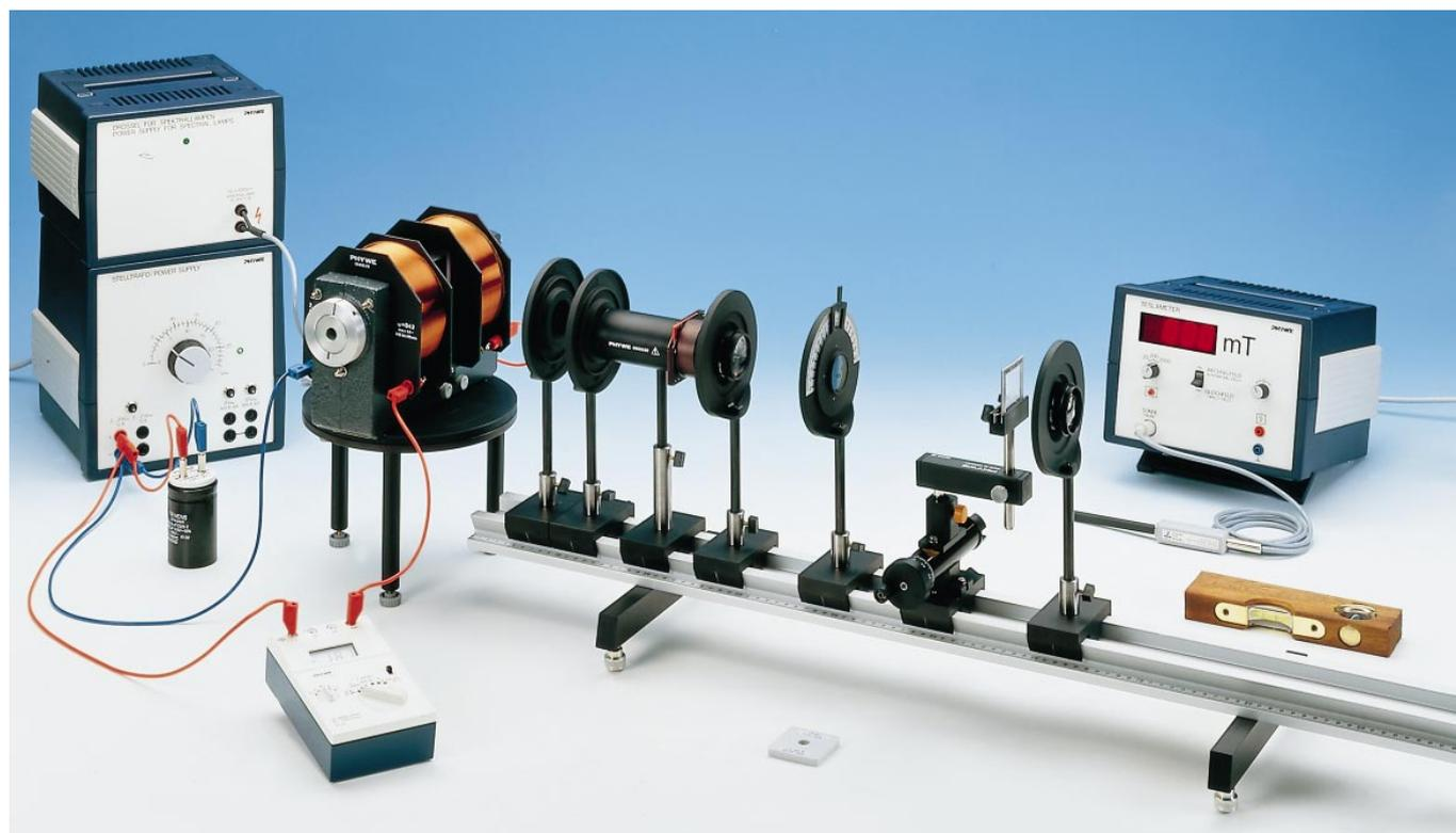
not move later on when the magnetic flux is established. The Cd-lamp is inserted into the gap without touching the pole-shoes and connected to the power supply for spectral lamps. The coils of the electromagnet are connected in parallel and via an ammeter connected to the variable power supply of up to 20 VDC, 12 A. A capacitor of 22 000  $\mu\text{F}$  is in parallel to the power output to smoothen the DC-voltage.
