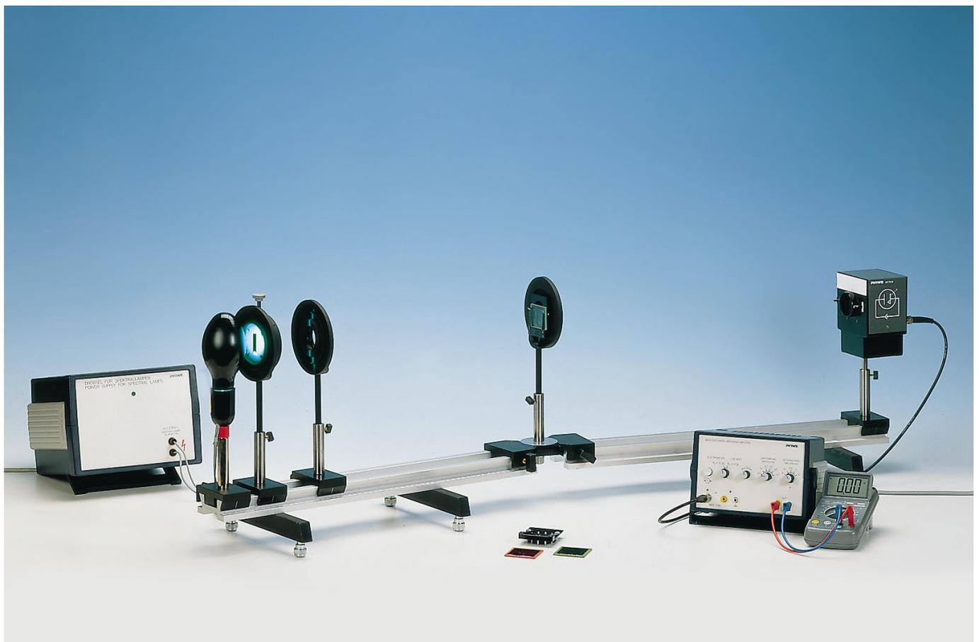
yellow and red spectral lines, place colour filters in front of the entrance diaphragm with the aid of an attachable diaphragm holder (525-nm coloured glass for the yellow spectral line and 580-nm coloured glass for the red spectral line)
