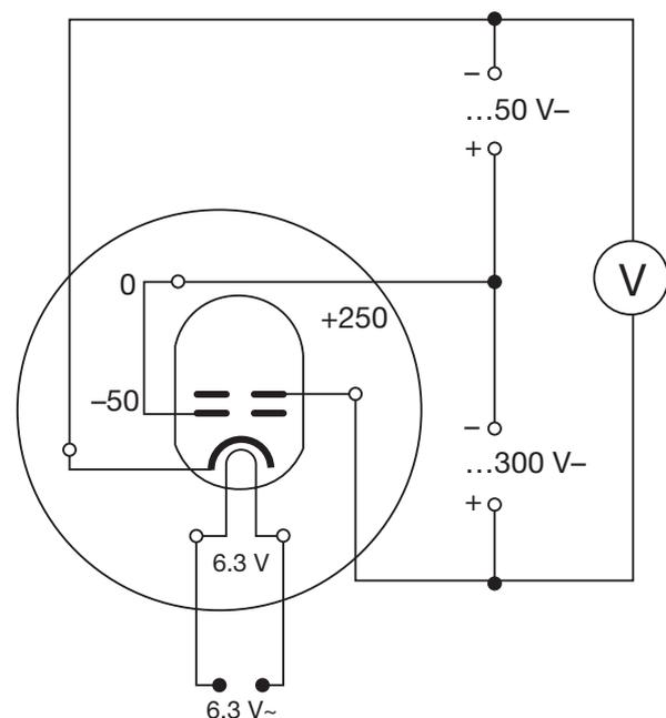
Fig. 3: Wiring diagram for Narrow beam tube.
