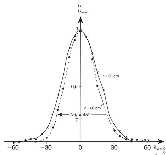
Fig. 3: Directional characteristic  $C_U(\vartheta, \varphi = 0)$  of the horn antenna in the polarization plane for different distances.
