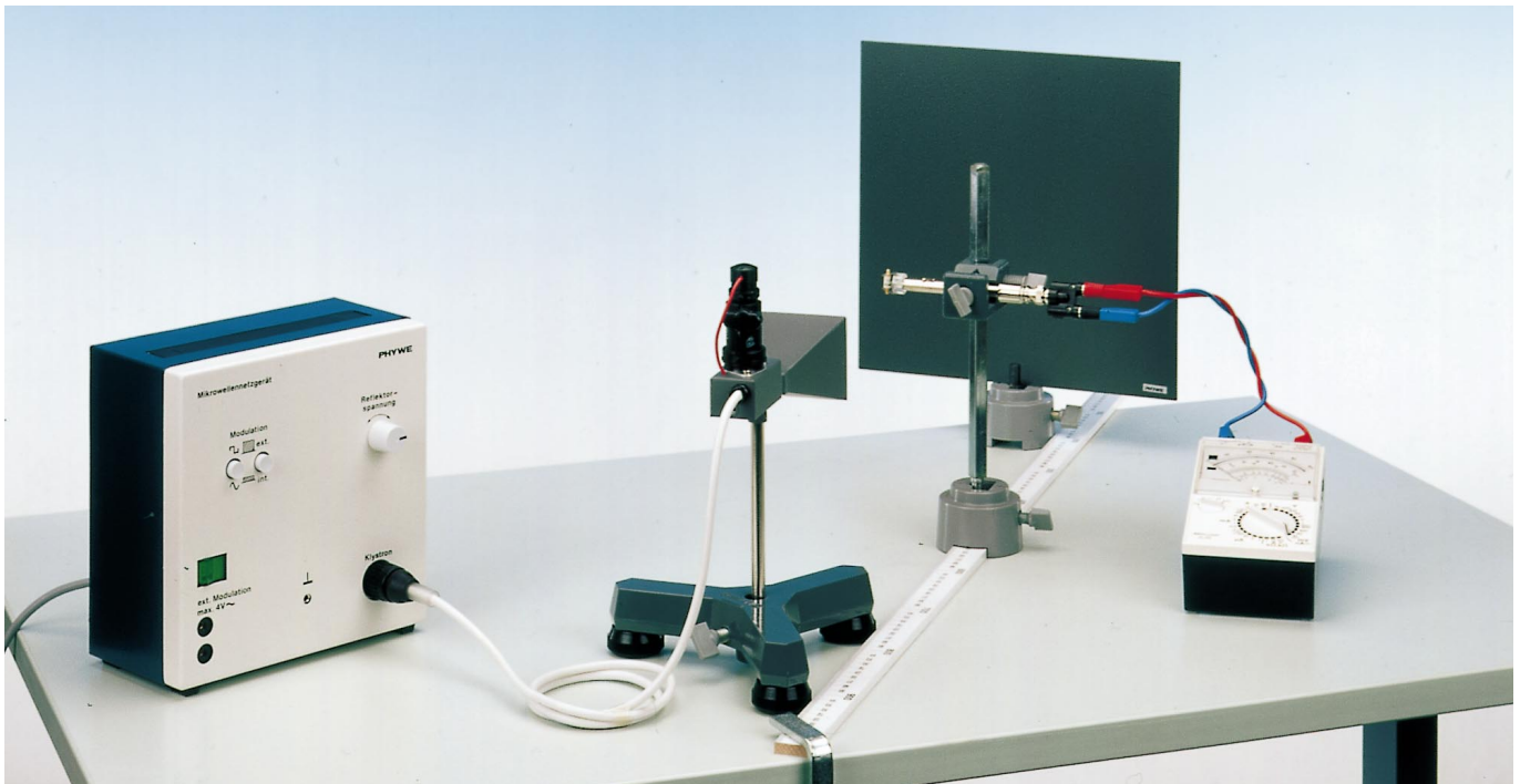
Fig.1b: Experimental set up for interference of microwaves with a plane parallel plate.
