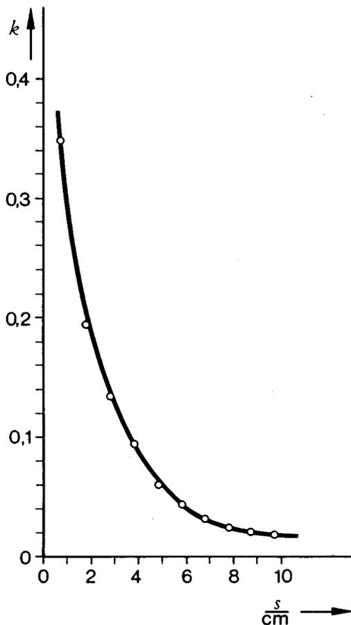
Fig. 8: Coupling constant as a function of the distance between the coils when the coupling is supercritical
