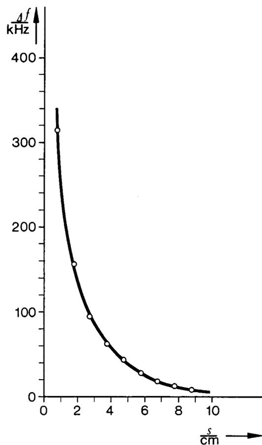
Fig. 9: Bandwidth as a function of the coil spacing.
