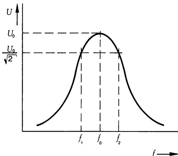
Fig. 3: Bandwidth of an oscillating circuit.
