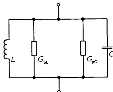
Fig. 5: Equivalent circuit of the parallel resonance circuit.
