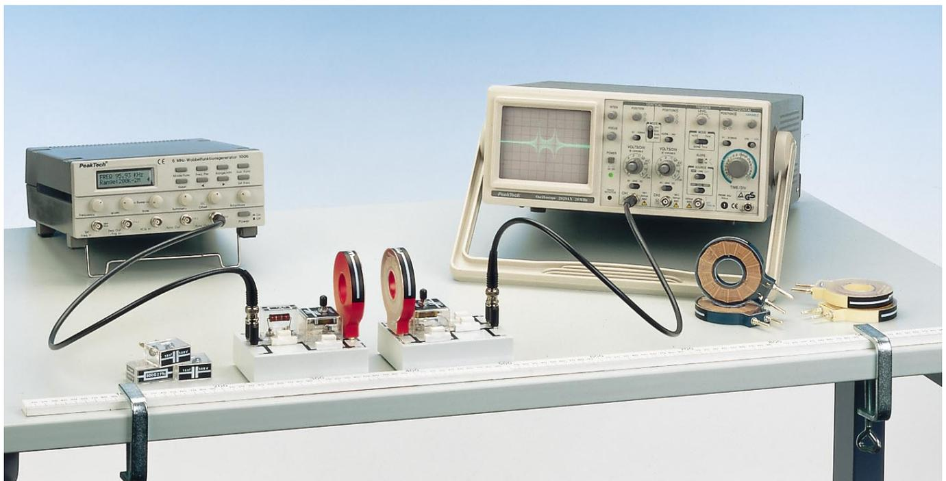
Fig. 2: Parallel oscillating circuit with series resistor  $R_s$ .
