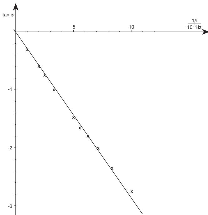
Fig. 6: capacitor and resistor in series,  $\tan \varphi$  as a function of  $1/f$ .
