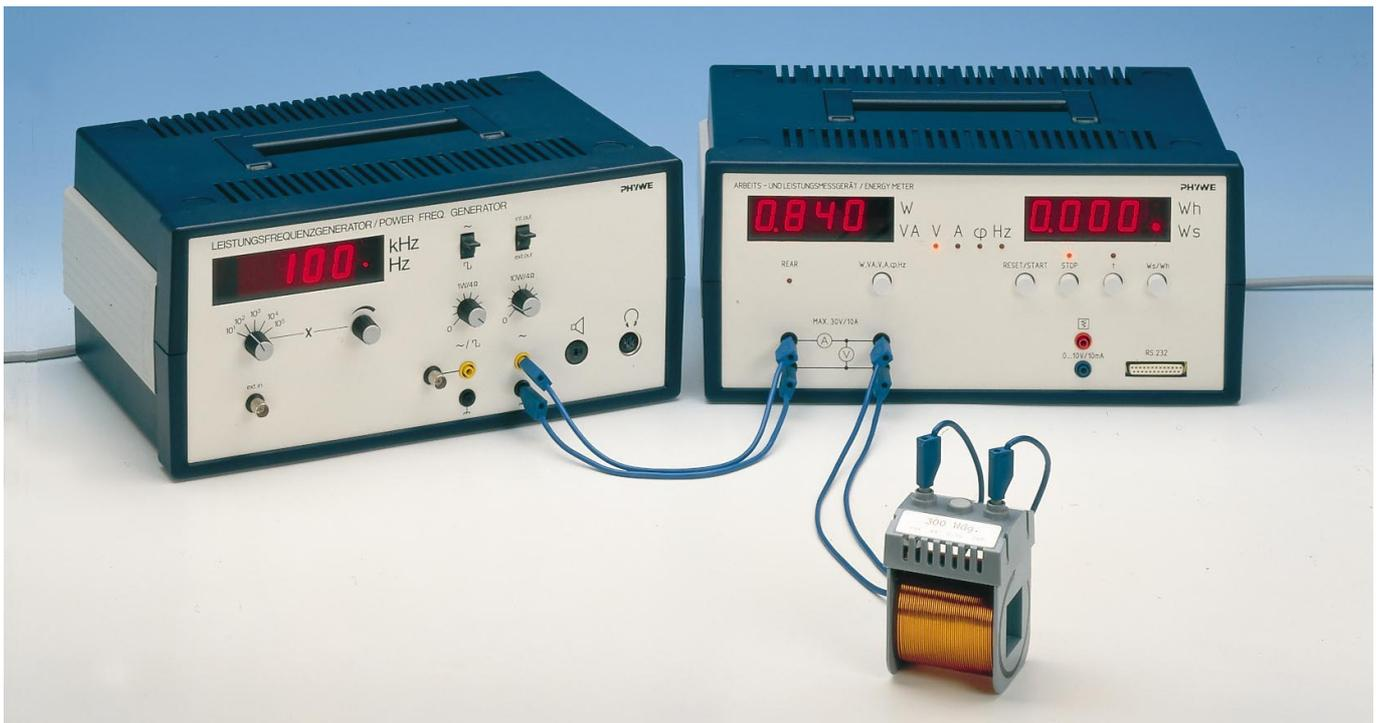
Fig. 2: self-inductance and resistor in series,  $Z^2$  as a function of  $f^2$ .
