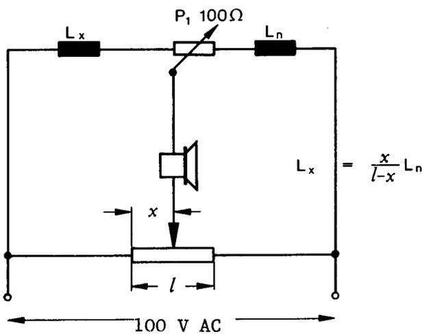
Fig. 3: Circuit for measuring inductances.
