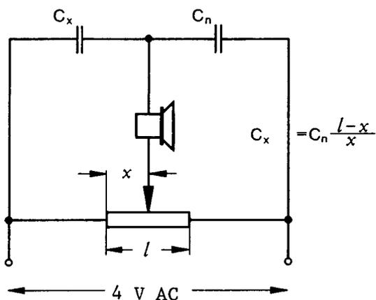
Fig. 4: Circuit for measuring capacitances.
