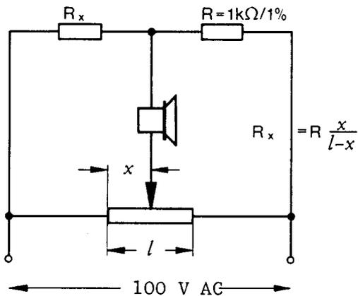
Fig. 2: Circuit for measuring resistance.
