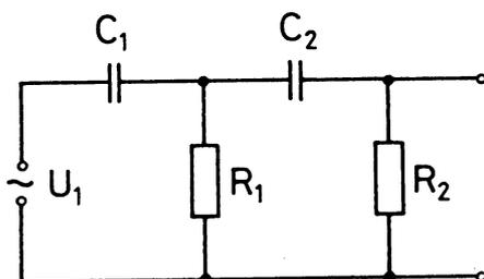
Fig. 3: Series connection of two CR networks.
