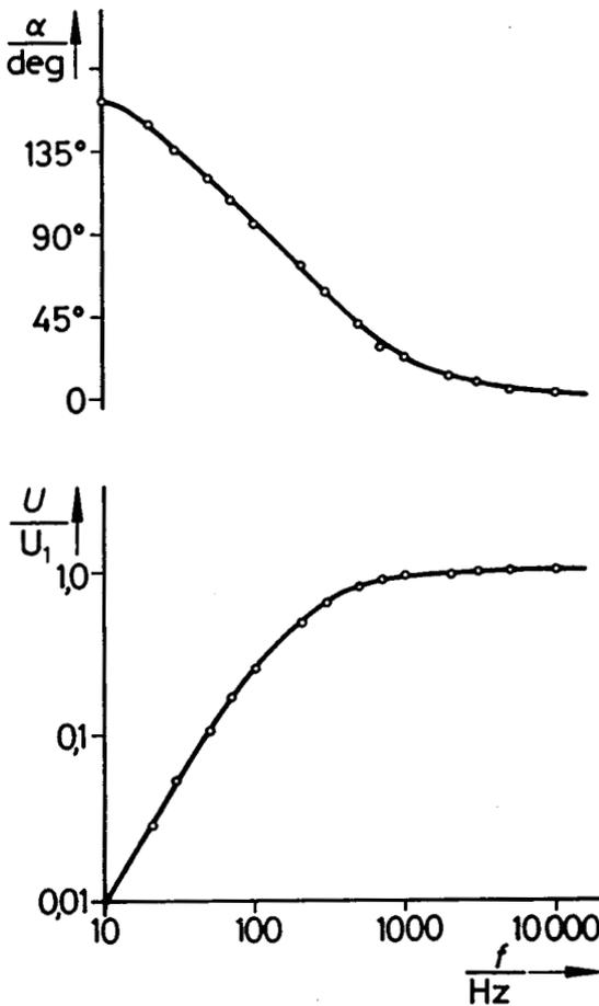
Fig. 6:  $U/U_1$  as a function of the frequency with the  $LR$  and  $RL$  network.
