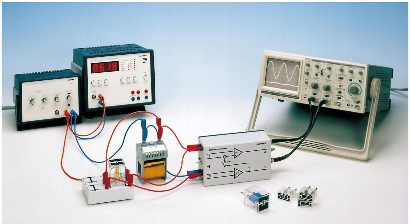
Fig. 2: RC/CR circuit.
