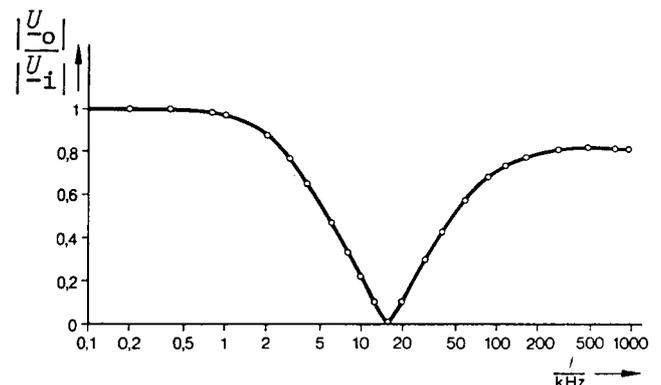
Fig. 10: Frequency response of the parallel-T filter.
