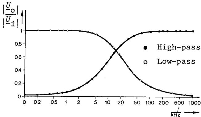
3. If we connect a high-pass and a low-pass filter together we obtain a band-pass filter. The following equation, with the abbreviation  $\omega RC = \Omega$ , applies to the unloaded circuit:
