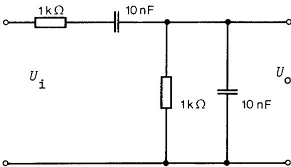
Fig. 4: Band-pass filter.
