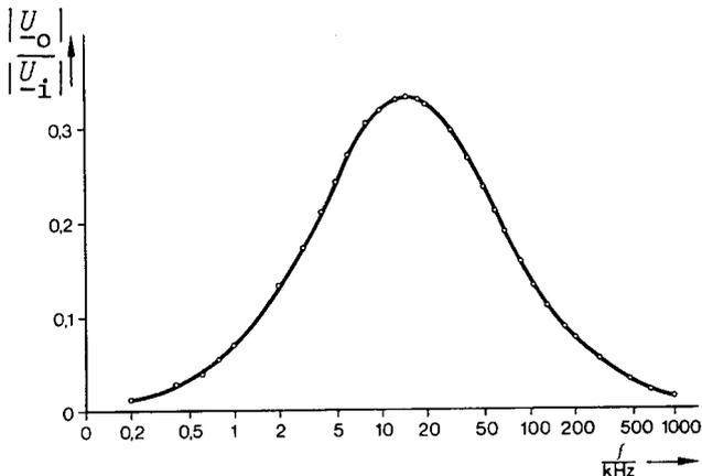
Fig. 8: Frequency response of the band-pass filter.
