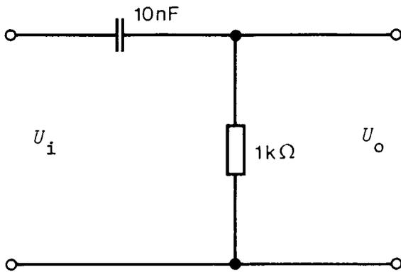
Fig. 2: High-pass filter.
