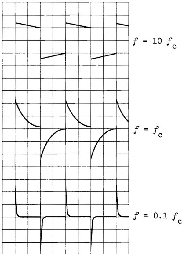
Fig. 12: Square-wave behaviour of the low-pass filter at various frequencies.
