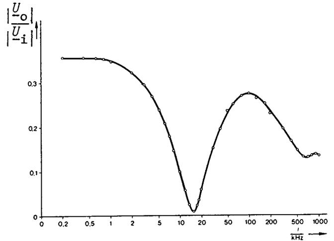
4. If we add a parallel-connected voltage divider consisting of ohmic resistors in the ratio 2:1 to the band-pass, we obtain a Wien-Robinson bridge:
