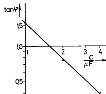
Fig. 7: Phase displacement ( $\tan \phi$ ) between total current and total voltage as a function of the capacitance.
