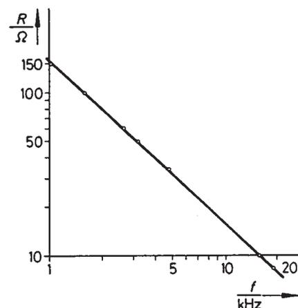
Fig. 3: Impedance of various capacitor as a function of the frequency ( $C = 1 \mu\text{F}$ ).
