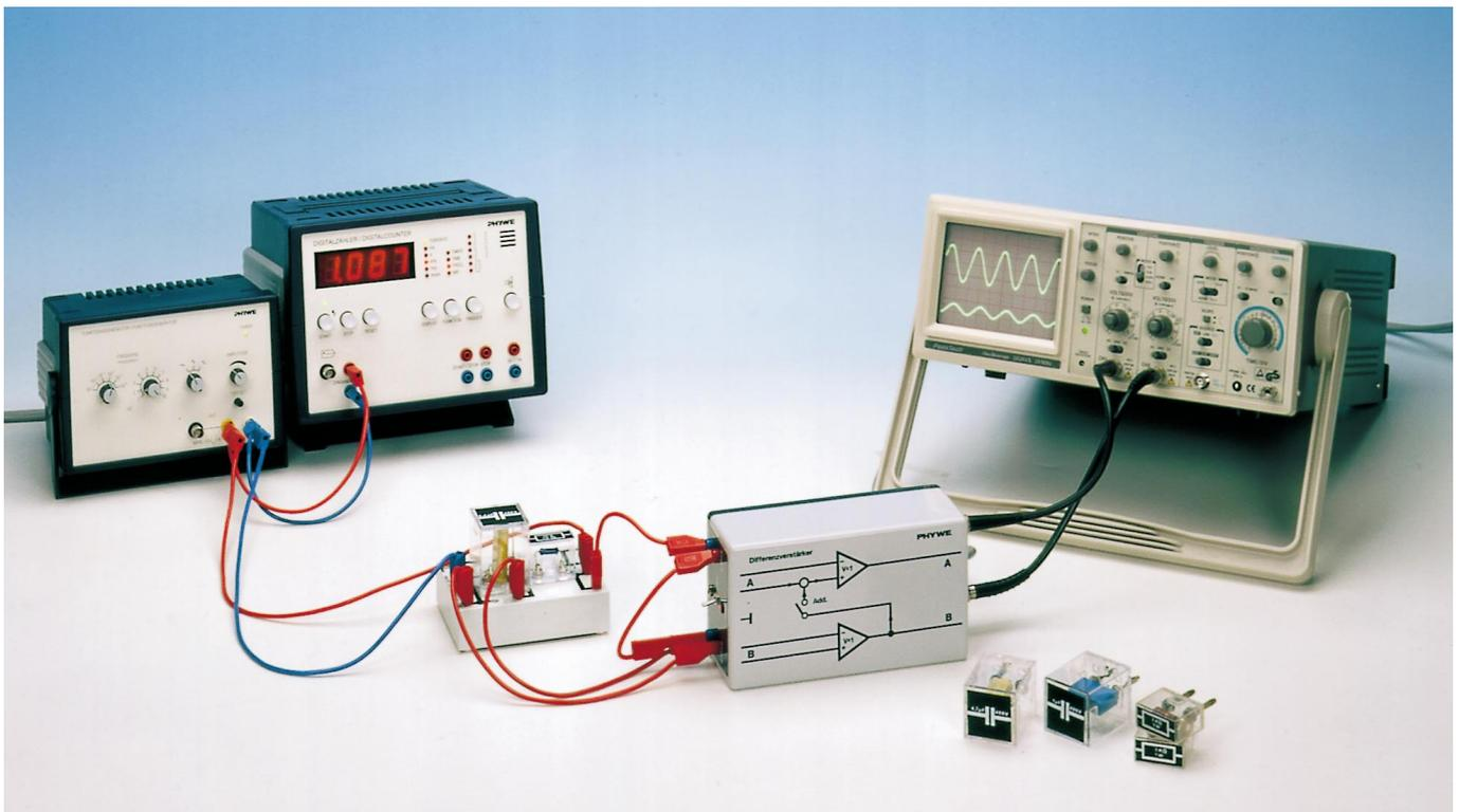
Fig. 2: Circuit for display of current and voltage with the oscilloscope.
