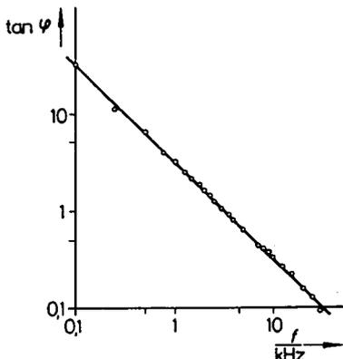
Fig. 5: Phase displacement ( $\tan \phi$ ) between total current and total voltage as a function of frequency.
