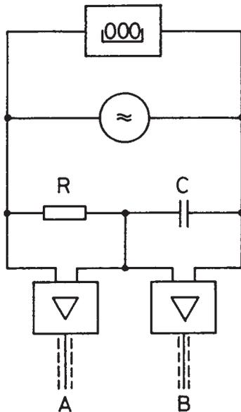
To determine the impedance of a capacitor as a function of the frequency, the capacitor is connected in series with resistors of known value. The frequency is varied until there is the same voltage drop across the capacitor as across the resistor. The resistance and impedance values are then equal:
