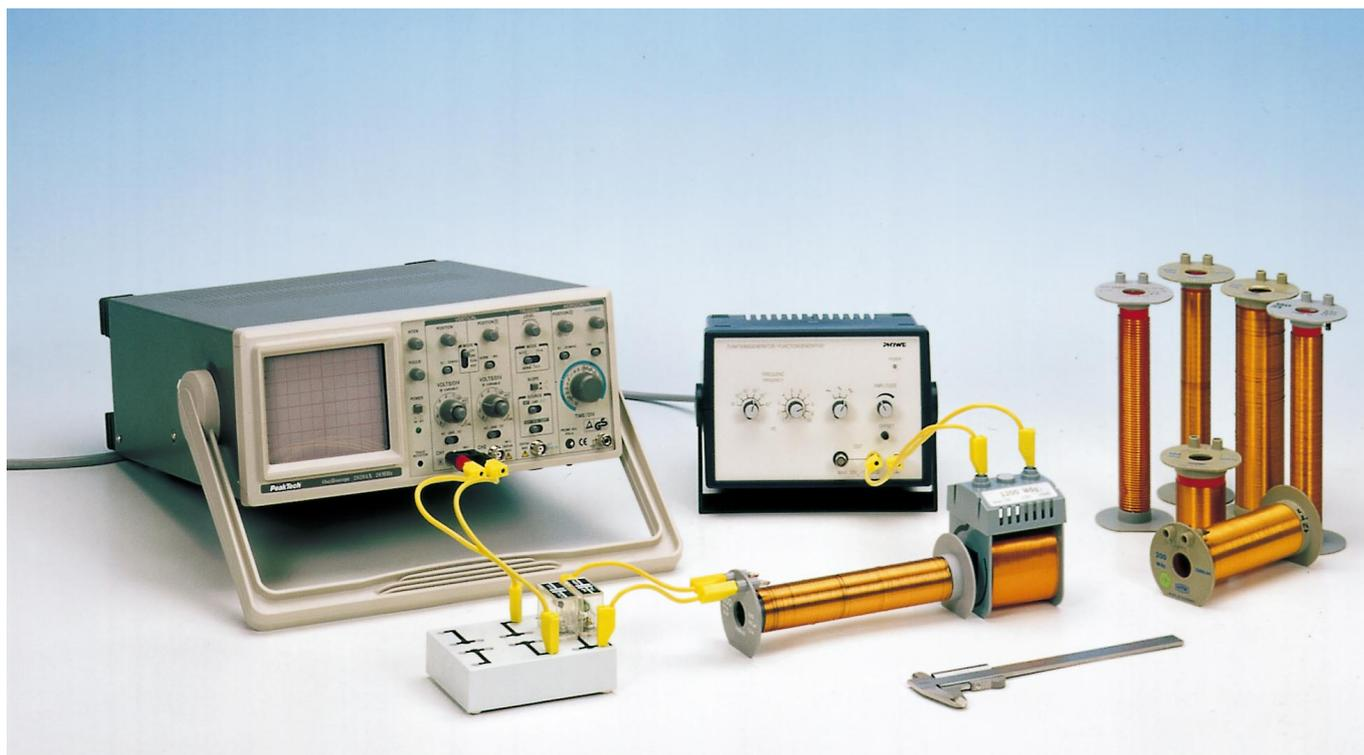
Fig. 2: Set-up for determining inductance  $L$ .
