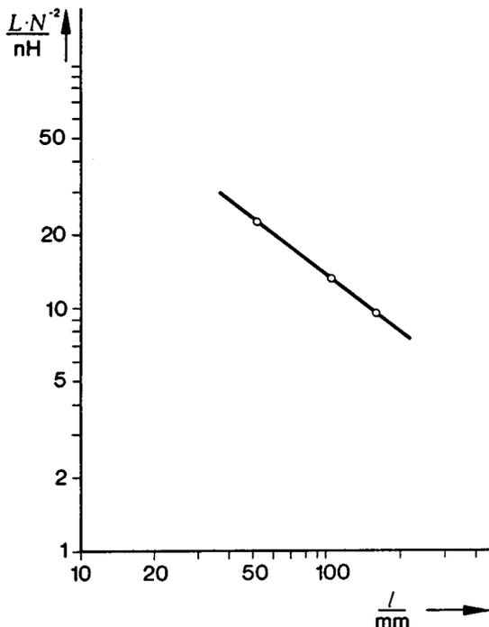
Fig. 5: Inductance per turn as a function of the length of coil, at constant radius.
