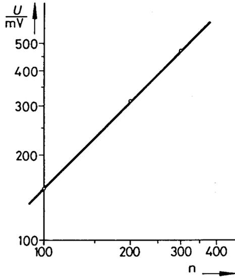
Fig. 5: Induced voltage as a function of the number of turns of the secondary coil with a primary current of 30 mA and a frequency of 10.7 kHz.
