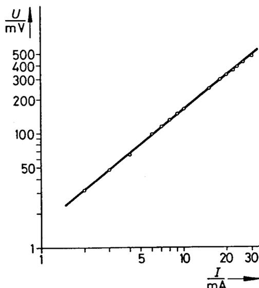
Fig. 2: Induced voltage as a function of the current in the primary coil at  $f = 10.7$  kHz, diameter of the induction coil  $d = 41$  mm.
