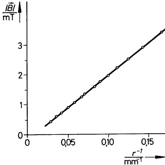
Because of the small zero-deflection due to the instrument and the effect of the other conductor and the “construction-kit” transformer, it is appropriate to carry out the measurement with small distances (up to approx. 3 cm) and with large currents (approx. 100 A).
