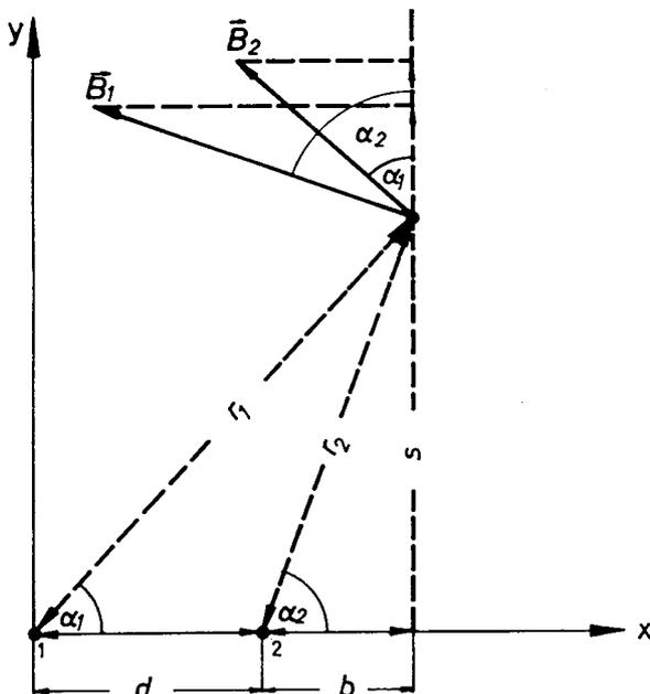
Fig. 5: Magnetic field of two conductors 1 and 2.
