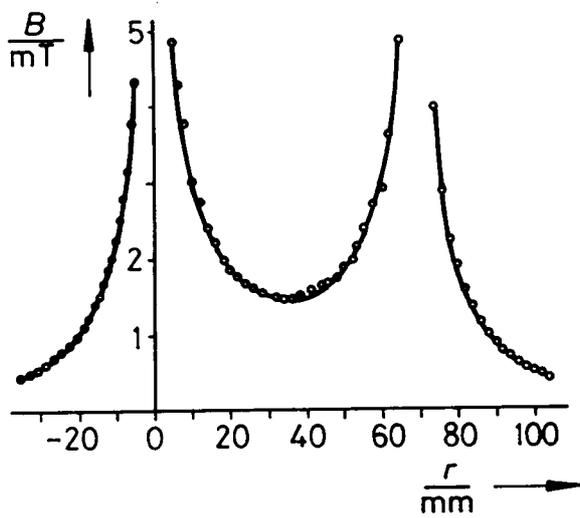
The strengthening of the fields can be clearly seen in the space between the two conductors, compared with the reduction in the area beyond the two conductors.
