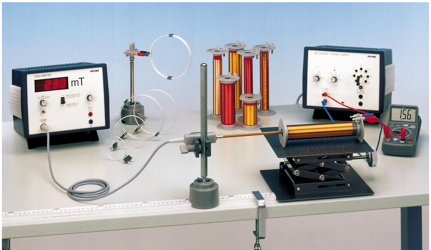
Fig.1: Experimental set-up for measuring a magnetic field.
