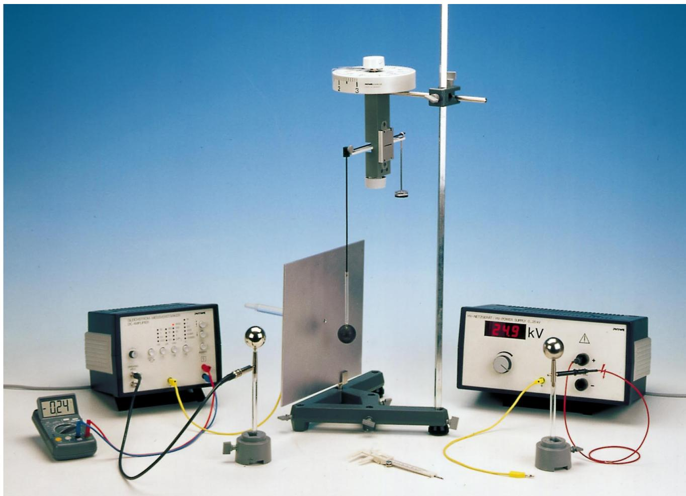
Fig. 2: Principle for Coulomb's law and image charge.
