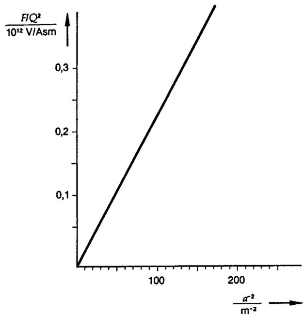
Fig. 5: Quotient of force  $F$  and square of the charge  $Q$  corresponding to the slopes of the straight lines in Fig. 6 as a function of the distance  $\alpha$  between ball and plate.
