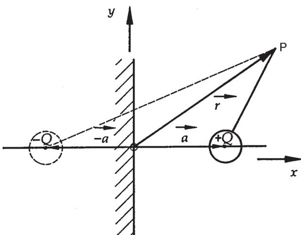
Fig. 3: Geometrical relationship in the plate/charge and image charge/charge system.
