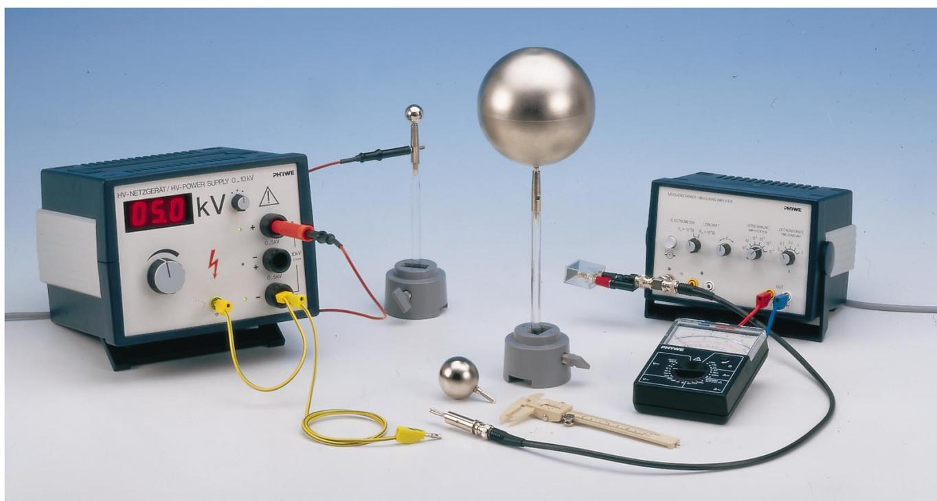
being charged anew, the test spheres must be discharged through contact with the free earth connecting cable.
