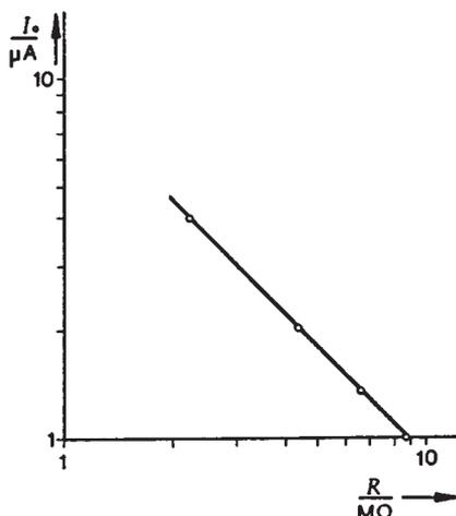
Fig. 8: Starting current  $I_o$  of the measured values in Fig. 6 as a function of the resistance.
