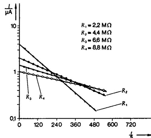
Fig. 6: Course of current with time at different resistance values; capacitance and voltage are constant at  $64\text{ }\mu\text{F}$  and  $9\text{ V}$  respectively.
