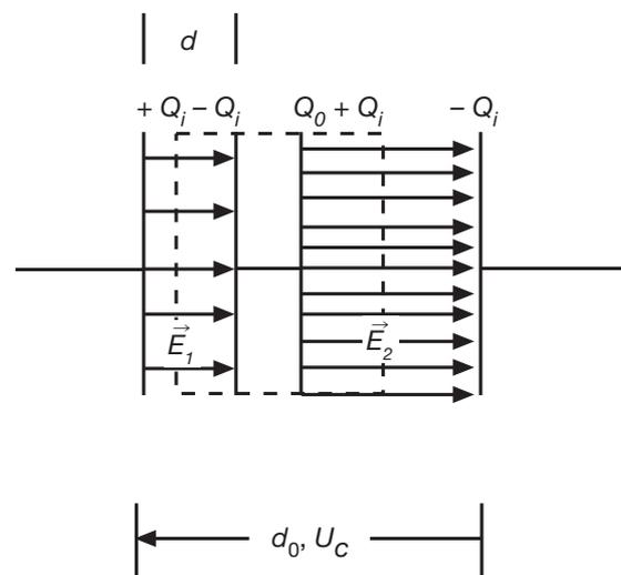
Fig. 3: Electric field and charges at the capacitor plates and at the transport plate. The dotted lines indicate the volume of integration.
