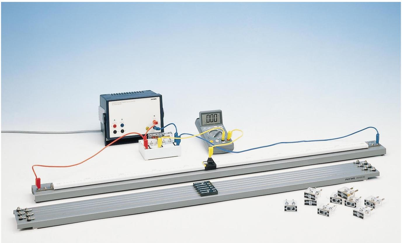
resistances of the connecting leads must be taken into account. Through the pilot light, the power unit is short-circuit-proof.
