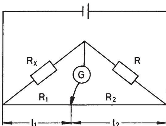
Fig. 2: Wheatstone bridge circuit.
