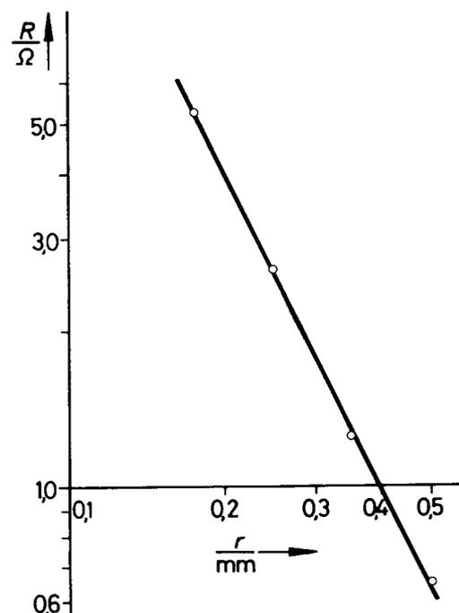
Fig. 3: Resistance of a conductor wire as a function of its radius  $r$ .
