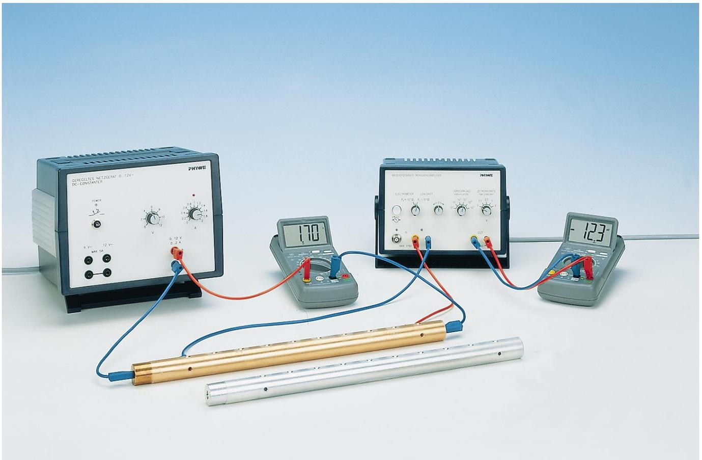
Fig. 2: Measuring the contact resistance and resistivity of connecting cords
