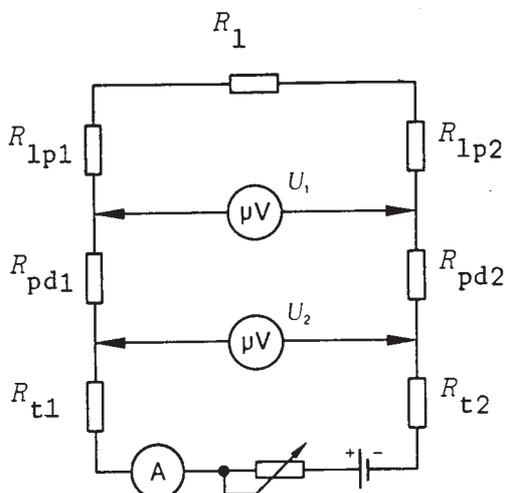
b) equivalent circuit diagram:  $R_t$ ,  $R_{pd}$  and  $R_{1p}$  are contact resistors,  $R_1$  a line resistor.
