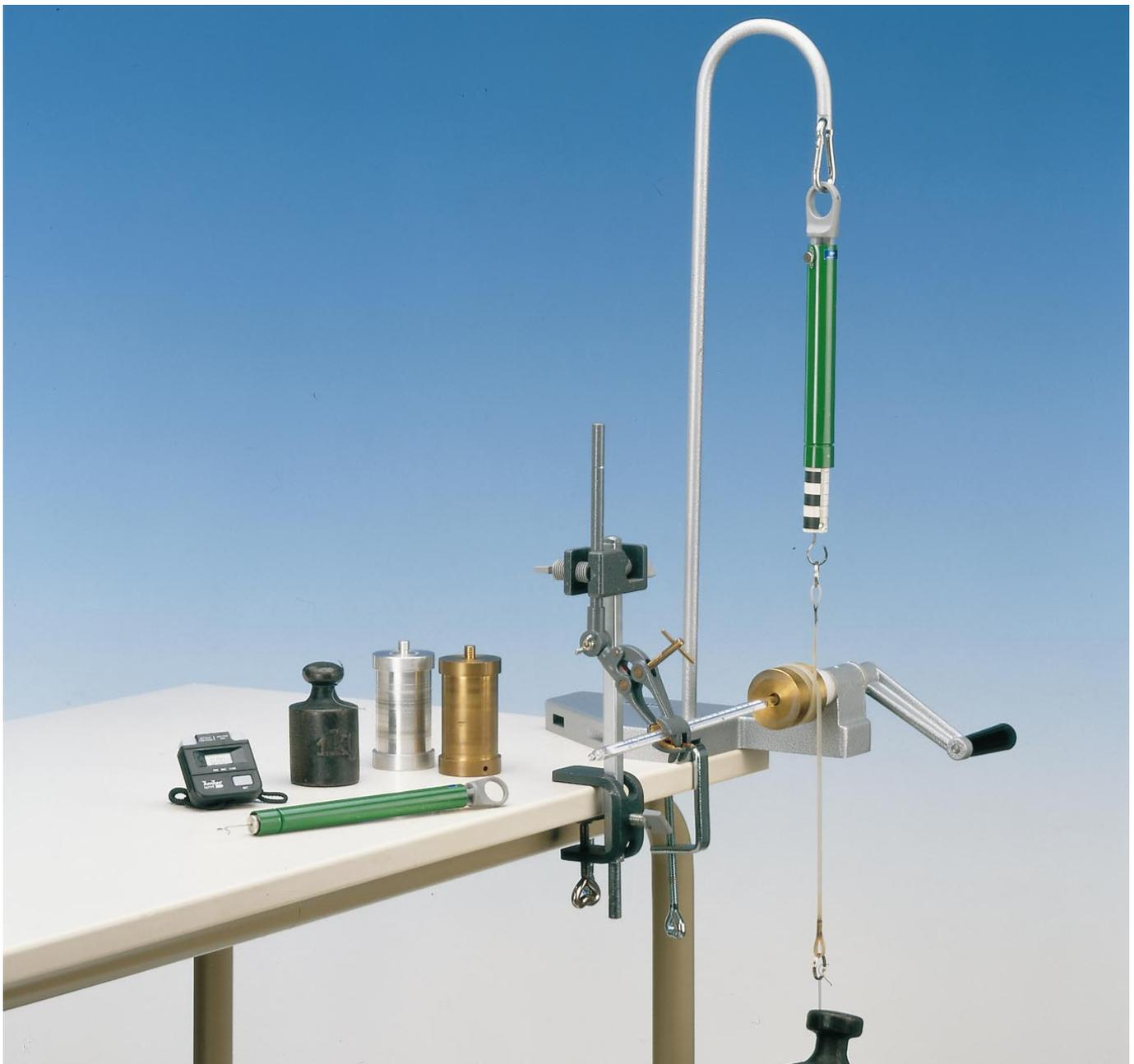
Fig. 2: Equilibrium of forces when the friction cylinder is rotated.
