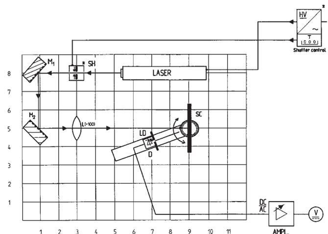
Experimental set-up for the qualitative verification of Lambert's Law of radiation (\* only required for 5 mW laser)
