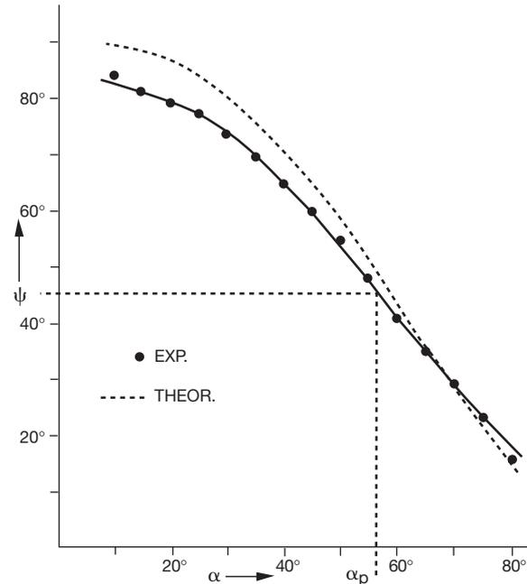
Fig. 7: Measured and calculated curves for the rotation of the direction of oscillation as function of the angle of incidence (azimuth of the incident beam is 45°).
