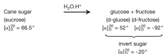
Fig. 2: Diagram of cane sugar inversion
