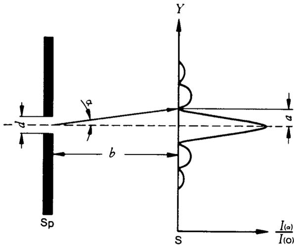
The principal maximum, and the first secondary maximum on one side, of the symmetrical diffraction pattern of a slit 0.1 mm wide (for example) are recorded. For the other slits, it is sufficient to record the two minima to the right and left of the principal maximum, in order to determine  $\alpha$  (Fig. 2).
