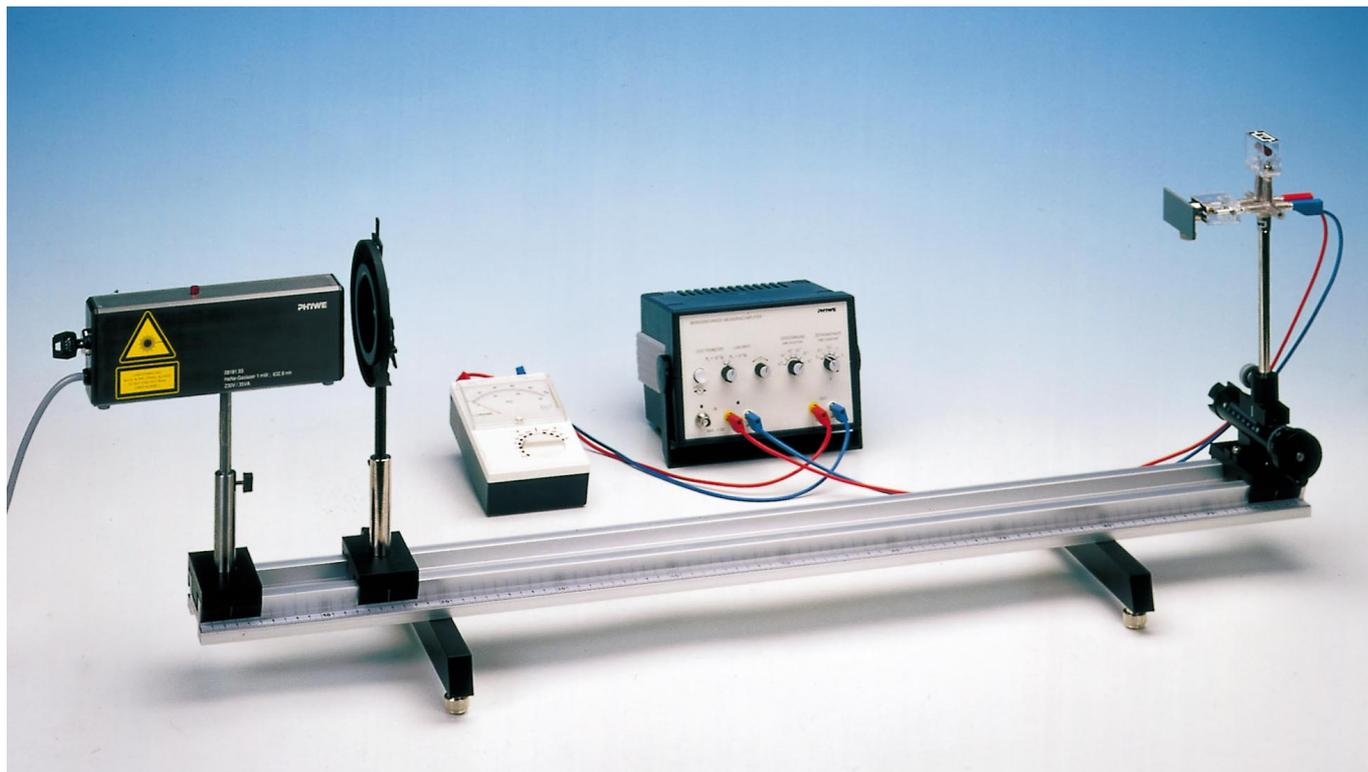
Fig. 2: Diffraction (Fraunhofer) at great distance (Sp = aperture or slit, S = screen).
