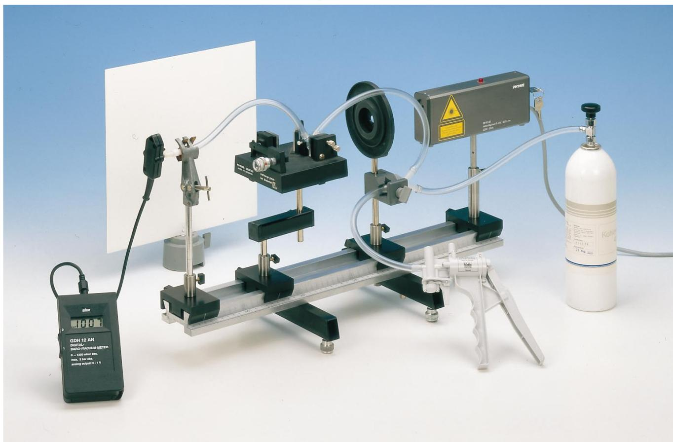
Fig. 2: Schematic representation of Michelson's set-up.
